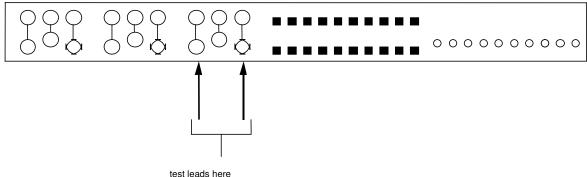
reading should be  $26 \pm .5$  ohms if not, adjust. pot. range 0-34 ohms
