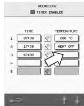
7. Enter the cavity temperature required on the keypad.
