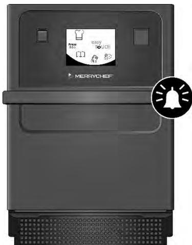
4. Wait for the cooking process to finish. An audible signal is given when the cooking process is finished. Follow the prompts displayed by the software.
