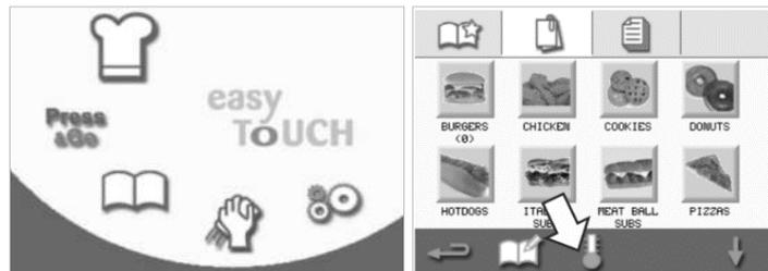
2. In the temperature screen, select the blue thermometer symbol to disable heating and start the cooling cycle.
