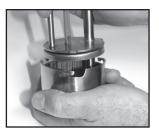
Remove bottom cap by twisting cap counter clockwise.
