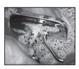
Wash and sanitize pump and components. Make sure to pump detergent and sanitizer through pump.
