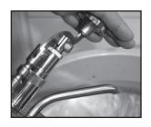
Remove pump from food container and pump out and dispose food product remaining in pump.
