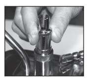
(Photo I) Unscrew set screw and remove lever. (Photo 2) Turn stem counter clockwise for a larger portion and clockwise for a smaller portion. Replace lever and set screw. Test the pump with the condiment to be dispensed and make additional adjustments if necessary.
