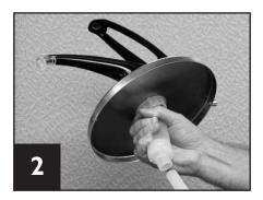
Disconnect the dip tube from the pump body by pulling the dip tube down using a twisting motion.
