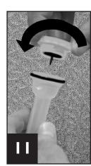
Unscrew the outlet valve and remove it from the plunger.
