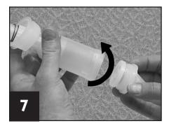
Unscrew and remove the pump bottom.
